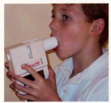
The Jones Satellite Spirometer is a versatile instrument. The lightweight, handheld device measures flow-volume and time-volume data. photo/courtesy the author
